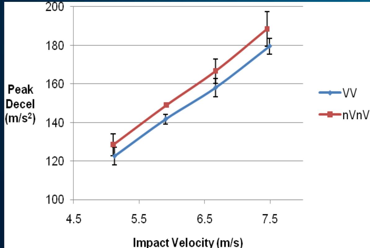
**Figure 7. Effects of venting on peak deceleration. Two pads, back to back. One pair is vented (VV). The other pair is not (nVnV). Standard deviation bars are shown (3-7 impact trials for each plotted data point for VV, 2-3 for nVnV).**
