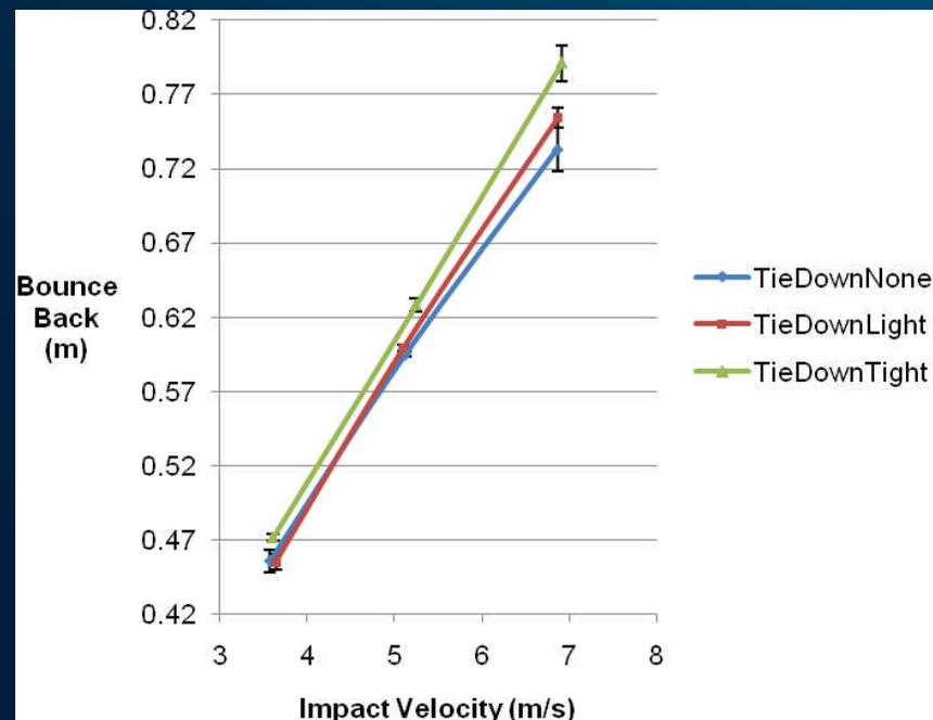
**Figure 8. Effects of front cover tightness on bounce back. Standard deviation bars are shown (2-3 impact trials for each plotted data point).**
