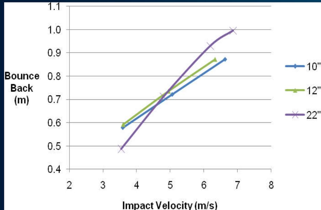
**Figure 3. Peak deceleration and bounce back with respect to pad thickness (42-45 lb open cell foam). The 22" pad was a combo of two pads (10" + 12").**
