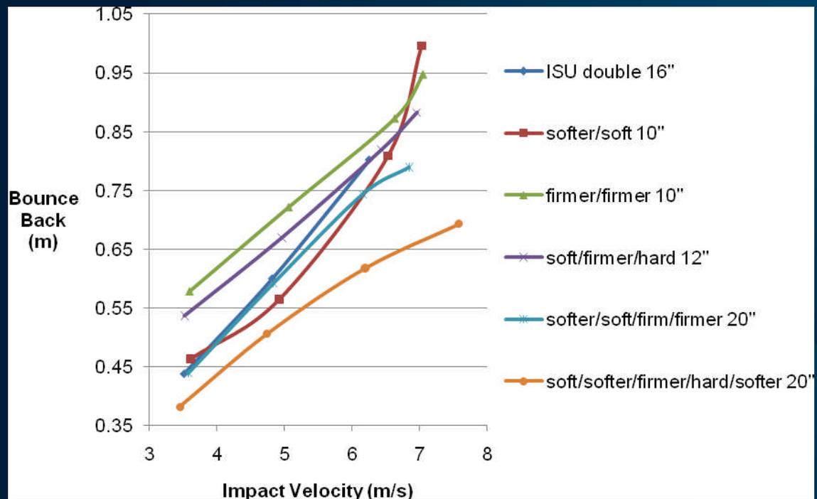
**Figure 4. Peak deceleration and bounce back for pads of various thicknesses with various layers of foam. Softer = 15 lb, soft = 26 lb, firm = 32 lb, firmer = 42 lb and hard = closed cell. All points represent the average of 2-6 impact trials. Standard deviations were less than 2% for bounce back, and less than 10 m/s<sup>2</sup> for peak deceleration.**
